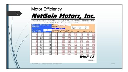
Slightly different motor, same spin direction but most efficient at a much lower RPM of 1087 and only about 72% efficient. This would be for a different type of vehicle and the motor should cost much less.
