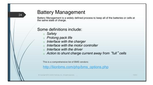
Cells or batteries in an EV are connected in series to increase voltage. Cells charged in series will deviate in relative state of charge over time. It is important to monitor each lithium cell and control the charge and discharge cycles to prevent cell damage or fires.
