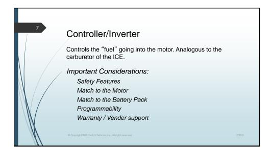
**Safety Features** – Since we are primarily concerned AC motors our primary concern is with the high voltage connections to the controller and from the controller to the motor. Are the connections sealed? Is the housing sealed, cooled?
