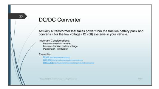
The DC to DC converter does the job of the alternator and must be sized in the same manner when determining the amount of watts are required for the low voltage system. For instance if you have a rather low demand, just headlights, running lights and a radio you would be able to use a 30amp DC to DC converter. If you added a 500 watt amp and a sub-woofer you would need a much higher output for your DC to DC converter.
