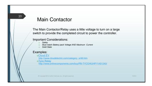
The purpose of the main contactor is to cut the power and de-initialize the vehicles energy supply. Normally I recommend opening the main contactor when the vehicle is powered off and closing the main contactor when charging or driving. This is a safety consideration so the pack voltage is minimized when the vehicle is not in use.
