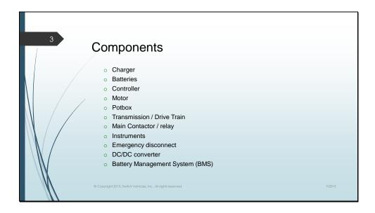
These are the 10 primary components installed in an electric vehicle.
