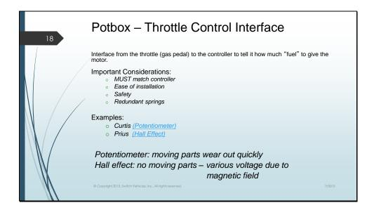
The potbox, "pot" is short for potentiometer, receives input from the driver, usually through the old gas pedal now called the accelerator pedal since we have no gas.
