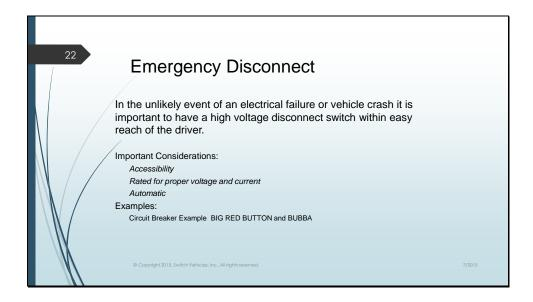
DC vehicles require an "Emergency Disconnect" it was described in detail when we discussed the Main Contactor. In a DC vehicle the emergency disconnect is usually a high capacity fuse opened when the driver pushes or pulls a lever. In an AC vehicle it is usually the main contactor.
